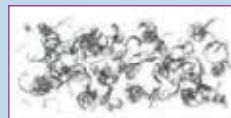
Thin chips which look like powder • Increase the feed or reduce the bandsaw speed.
